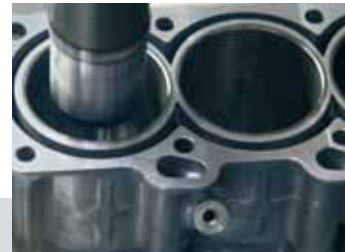
PCBN insert Cylinder boring (rough & finish)
